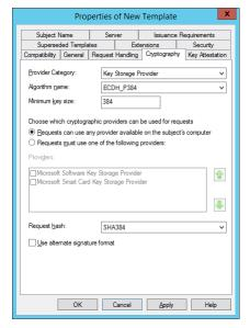
When configuring the templates for issuance within MyID, you must select an ECC type of the appropriate size from the **Key Algorithm** drop-down list; for example for an **ECDSA\_P384** or **ECDH\_P384** certificate template, select **ECC P384** from the **Key Algorithm** drop-down list.
